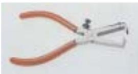
Very popular but success depends upon the operator setting the tool properly, furthermore the tool must be adjusted each time a different type of wire has to be stripped.
