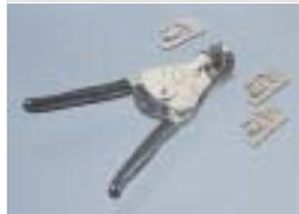
These tools feature precision ground die blades against which the wire insulation is further supported and guided. The tools at right are each individually specified to specific wire size and insulation width. The tools below right can strip a number of wire sizes but each die nest is also designed for a specific wire size and insulation width. These tools are especially suitable for fibre optic and aerospace wires and cables.
