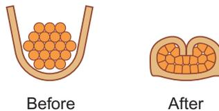
This process requires that the middle of the conductor barrel is sectioned with a precision wet saw, mounted in a mould or fixture, ground and then polished. The section may further be chemically etched to enhance detail.
