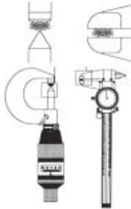
For high precision applications it may be necessary to produce a cross-section of the crimp area to further assess its efficacy.
