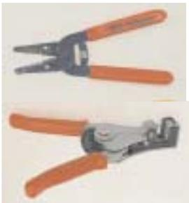
These tools feature ground nests into which wires can be placed for stripping. Whilst useful as service tools they can be easily misused. Success relies on the operator putting the right wire into the right nest. All too often in production this does not happen. Furthermore a large range of tools are required to cover a reasonable wire size range.
