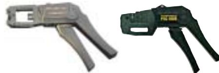
One of the principal drawbacks of scissor action crimp tools is that the connector is always to some degree squeezed towards the front of the tool. Tool manufacturers design dies to allow for this effect, yet there will always be
