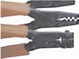
These tools employ a compound plier action to increase leverage and therefore increase the force that can be applied at the dies. However the crimp result is still directly related to the hand force applied. Over Centre/Toggle Action Crimp tools
